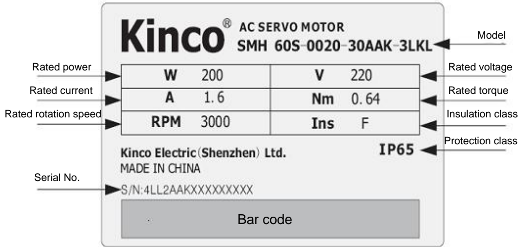
Fig. 1-2 Nameplate of a servo motor
