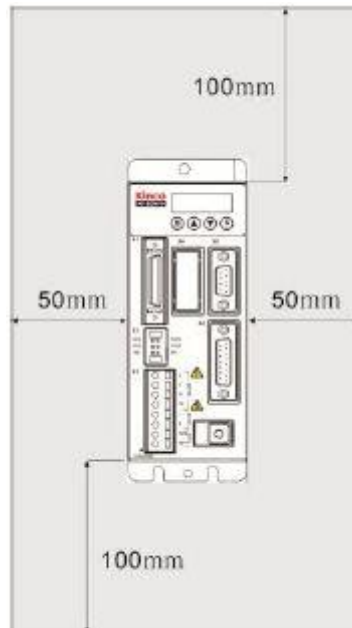
Fig. 2-1 Installing a servo driver
